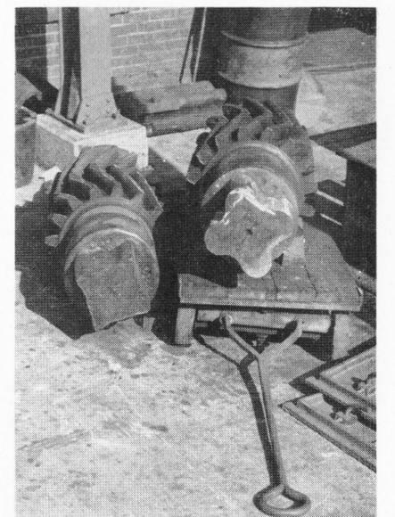
These herringbone pinion gears which were badly worn on the ends were restored to original usefulness by electric welders. Scallops on the gear on the truck were re-built. The one on the ground has not been repaired as yet, and is waiting attention of the welders.
